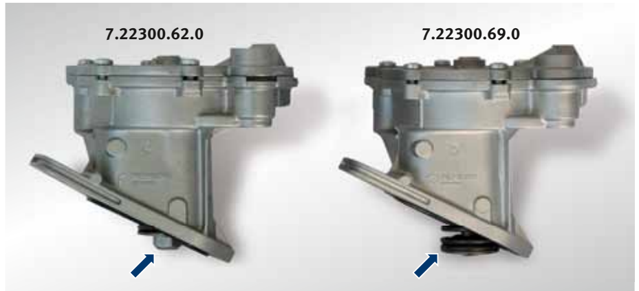
Fig. 2: Vacuum pump comparison
