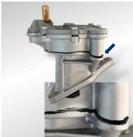
Fig. 1: Broken pump casing
