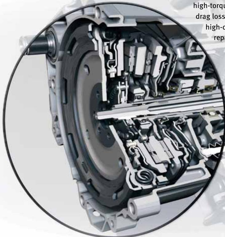
Like conventional single-disc clutches the dry double clutch of the 7-speed DCT is also located in the gear-box housing. There are no drag losses as it is not oil-immersed, which increases engine and fuel efficiency compared to wet double clutches. It also makes repairs less complex.
